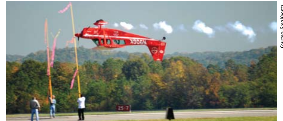
There are some maneuvers that demand help from an inverted system, including prolonged inverted flight.
