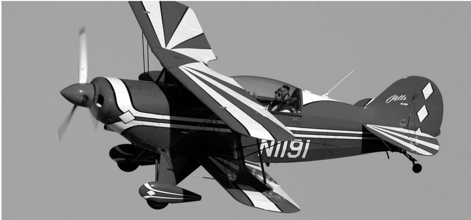
Mastering uncoordinated flight will improve forward visibility in blind airplanes such as the Pitts. Robert Bismuth.
