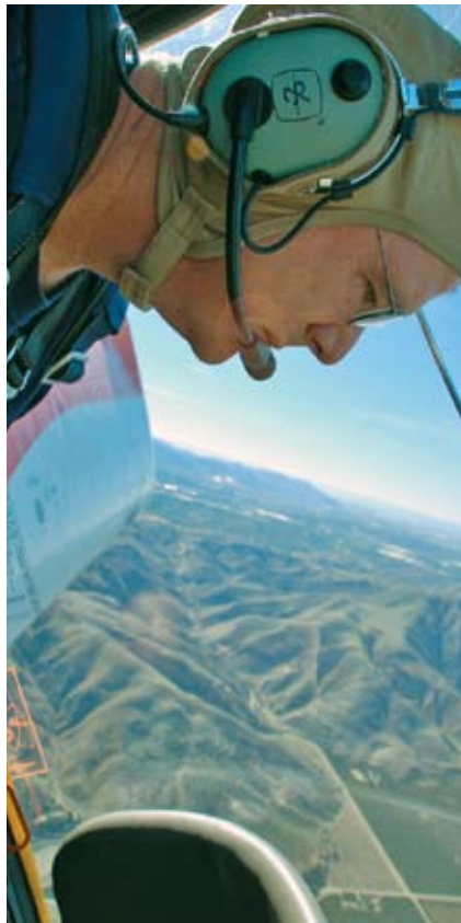
The Zlin 242L Post-Spin Attitude is 60-65 Degrees Nose-Down
